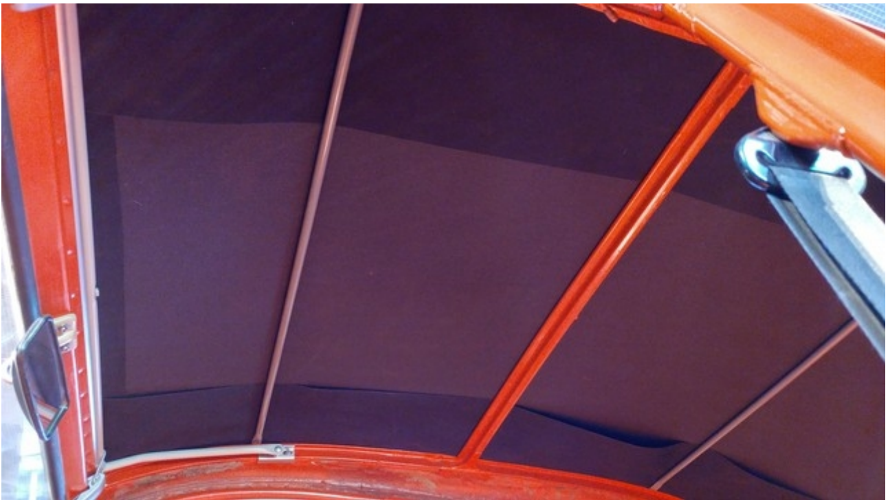
Picture shows supporting bars roughly in place, sides sat how they should be, well onto the body with no lifting.
