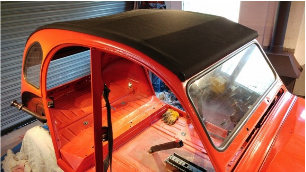
Picture shows supporting bars roughly in place, sides sat how they should be, well onto the body with no lifting.
